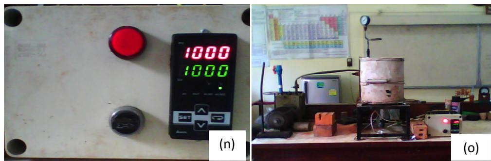
Figure 2. Photographs of the (n) DELTA A Series Temperature Controller DTA4896 at  $1000^{\circ}\text{C}$  and (o) experimental setup of sample preparation system
